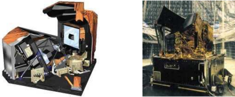
Figure 3.4. Artist impression of the GOMOS instrument (left panel). The GOMOS instruments before transportation from Matra Marconi Space in Toulouse to the test facility in Liege. The instrument is mounted on a stand with the optical unit on the top and the instrument electronic panel below, in basically the same configuration as on the spacecraft (right panel) ( http://envisat.esa.int , July 2004).
