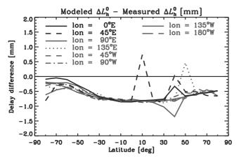
**Figure 2.** Difference between modeled (equation (12)) and "true" (realistically simulated) zenith hydrostatic delays for eight meridionally oriented chains of stations with  $10^{\circ}$  spacing for Sept. 15, 1999, 12UT (the absolute delay  $\Delta L_h^0$  at sea level is  $\sim$ 2.3 m).
