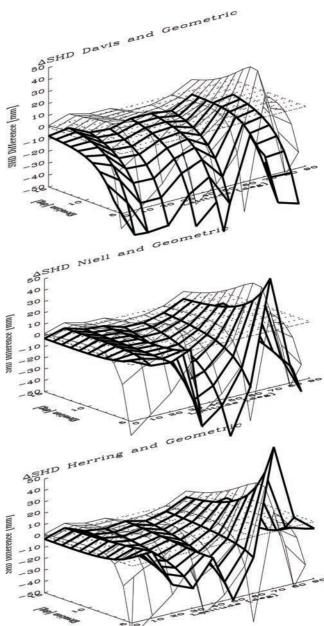
**Figure 3.** Differences between modeled and "true" slant hydrostatic delays for Sept. 15, 1999, 12UT, 45°E. The "geometric" mapping function (light-lined grid) is compared to the Davis (top), Niell (middle), and Herring (bottom) mapping functions (bold-lined grid), respectively.
