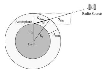
**Figure 1.** Schematic illustration of the construction of the "geometric" mapping function.
