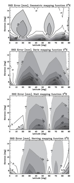
**Figure 4.** Differences between modeled and "true" slant hydrostatic delays for Sept. 15, 1999, 12UT, 0°E, using the "geometric" (top), Davis (upper middle), Niell (lower middle), and Herring (bottom) mapping function, respectively.
