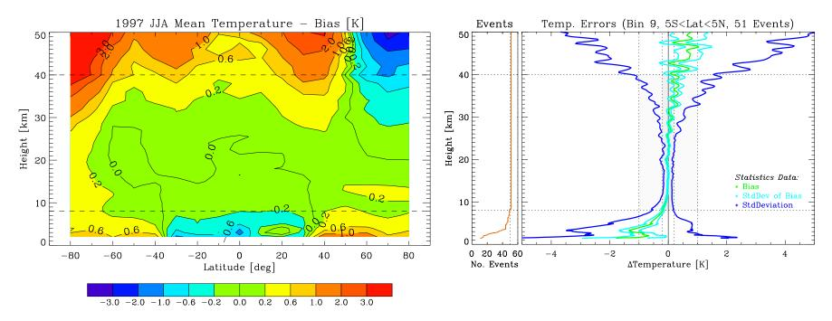
Illustration of retrieval performance using GNSS-LEO occultation data (realistic end-to-end simulations; *left:* lat-height slice of temperature errors of ~50 profile mean, *right:* vertical error structure at equator)
