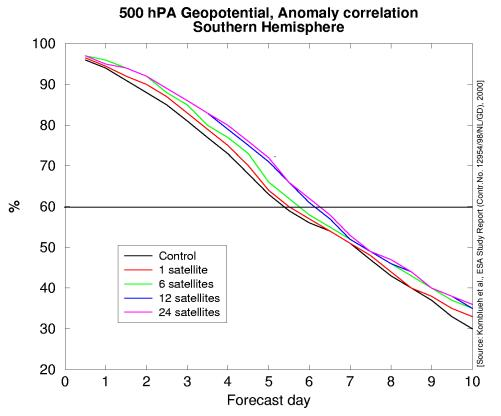
Forecast skill improvement due to GNSS-LEO data from ACE+-like constellations (1, 6, 12, 24 LEO satellites; *Control:* no ingestion of GNSS-LEO data)
