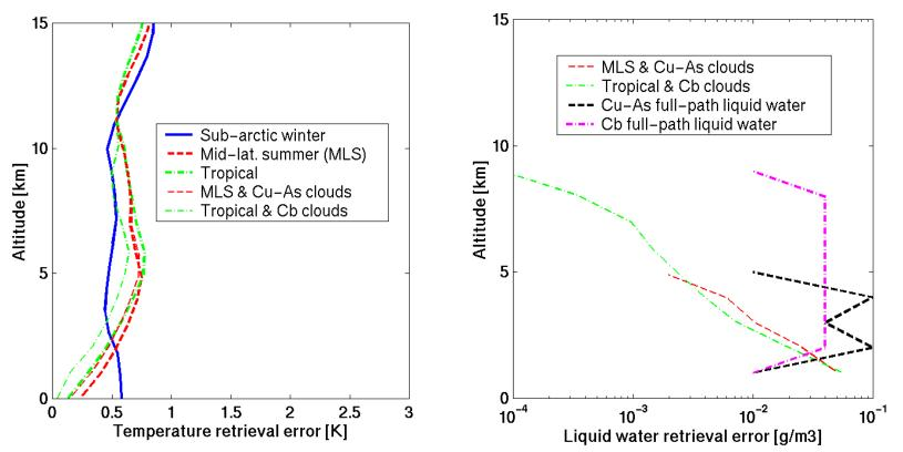
Illustration of temperature and liquid water retrieval performance for LEO-LEO occultations (realistic sensor errors, moderate cloudiness, no horiz. variability)
