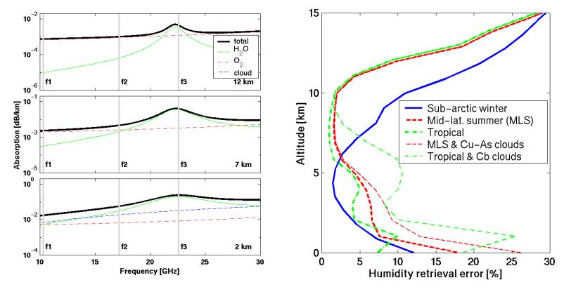
Illustration of absorption properties and humidity retrieval performance for LEO-LEO occultations (realistic sensor errors, moderate cloudiness, no horizontal variability)
