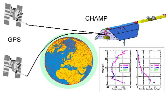
Figure 2. Schematic view of the CHAMP RO experiment and indication of the temperature and humidity retrieval performance (lower-right inset) based on an occultation event from the very first measurement day on February 11, 2001 (graphics: J. Wickert/GFZ Potsdam).
