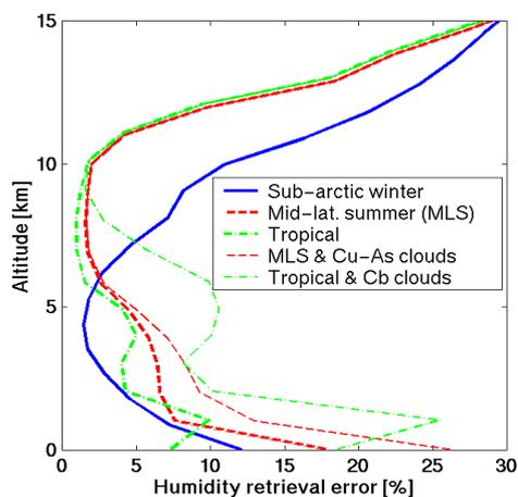
Figure 3. Specific humidity retrieval errors obtained for realistically simulated LEO-LEO RO measurements (adopted measurement noise and gain drift consistent with the ACE+ LEO-LEO RO sensor specifications). Several cases based on different standard atmosphere profiles and different cloud conditions are shown; the vertical resolution involved (estimated via “averaging kernel width” and “Backus-Gilbert spread”) is  $\sim 1$  km.
