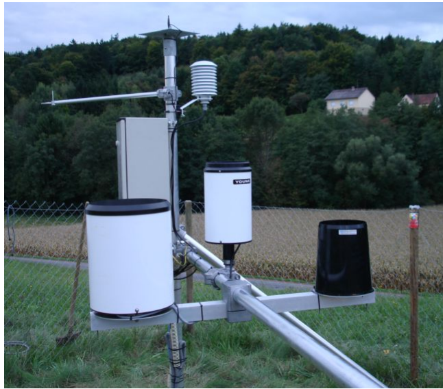
Figure 5.1.: Precipitation measurement systems at the reference stations. From left to right: Kroneis MeteoServis, R.M. Young, Theodor Friedrichs & Co.
