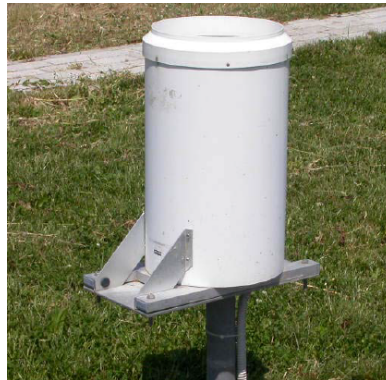
Figure 4.6.: Tipping bucket rain gauge model AP-23 from Anton Paar (Vuerich et al. [2009]).
