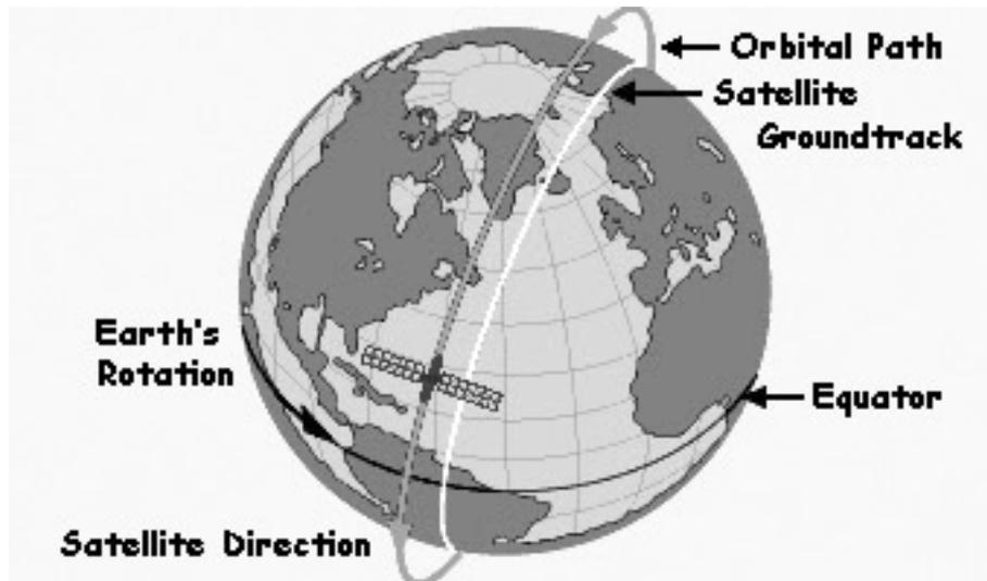
**Figure 3.5:** Orbital path of a NOAA satellite. For one orbit it needs approximately 103 min. During that time the Earth rotates about  $25.7^\circ$  eastward. There follow 14 orbits per day <http://www.crisp.nus.edu.sg/~research/tutorial/spacebrn.htm>.
