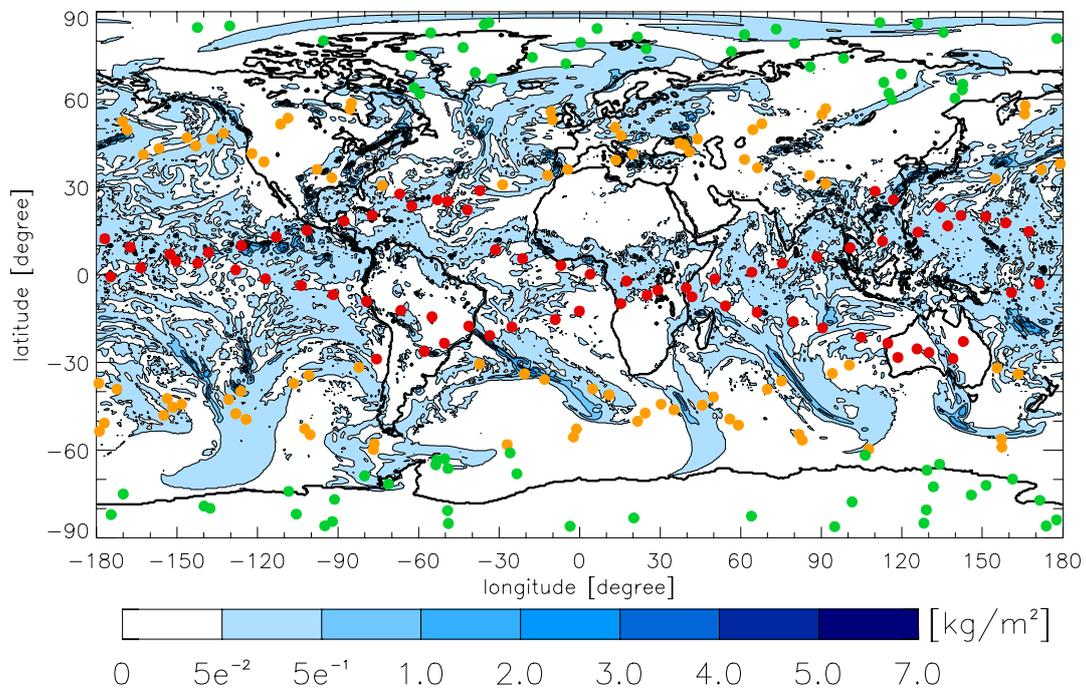
**Figure 3:** Coverage with 1 day of ACE+ LEO-LEO RO events, sorted into low (red dots), middle (orange dots), and high (green dots) latitude bands of 30 deg width each. The background shows the vertically integrated liquid water density (units kg/m²), indicating cloud coverage (data from the Sept 15, 2002, 12 UT, ECMWF T511L60 analysis). [from Kirchengast et al., 2004c]
