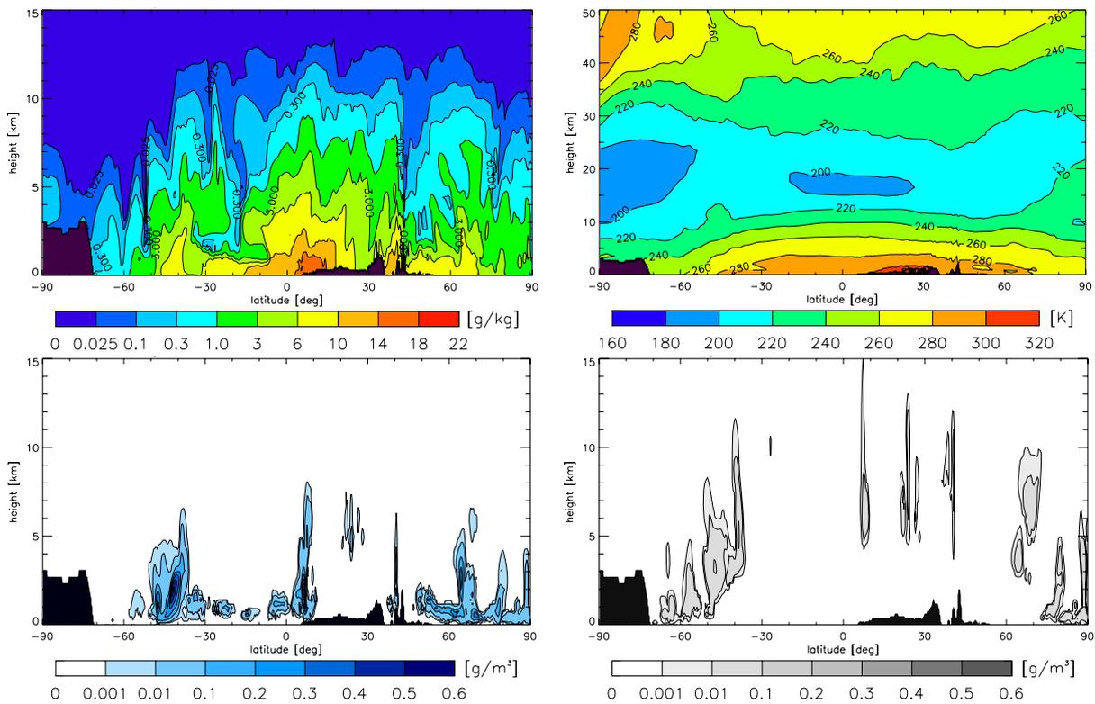
**Figure 2:** Specific humidity (top-left), temperature (top-right), liquid water density (bottom-left), and ice water density (bottom-right) latitude-height cross sections at 0 deg longitude through the ECMWF T511L60 analysis of Sept 15, 2002, 12 UT, used in the simulations. [from Kirchengast et al., 2004b]
