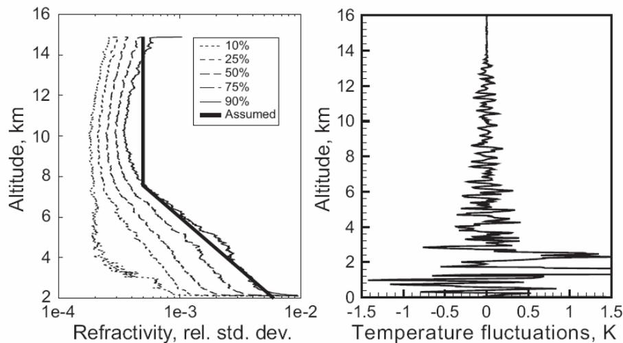
**Figure 5:** (left) Profiles of turbulent fluctuations (rms) on the basis of a dataset of high-resolution radiosonde profiles observed at the low latitude station St.Helena (15.6°S, 5.4°W): Median profile (50%) and different percentiles. The profile “Assumed” (heavy black line), meant roughly to reflect the upper decile (90%), is the one used for the turbulence modeling. (right) associated turbulent fluctuations in the dry temperature. [from Gorbunov and Kirchengast, 2005; adapted]
