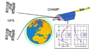
Figure 2. Schematic view of the CHAMP RO experiment and indication of the temperature and humidity retrieval performance (lower-right inset) based on an occultation event from the very first measurement day on February 11, 2001 (graphics: J. Wickert/GFZ Potsdam).
