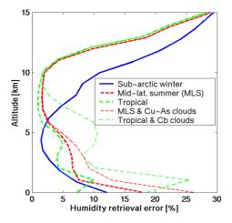
Figure 3. Specific humidity retrieval errors obtained for realistically simulated LEO-LEO RO measurements (adopted measurement noise and gain drift consistent with the ACE+ LEO-LEO RO sensor specifications). Several cases based on different standard atmosphere profiles and different cloud conditions are shown; the vertical resolution involved (estimated via "averaging kernel width" and "Backus-Gilbert spread") is ~1 km.
