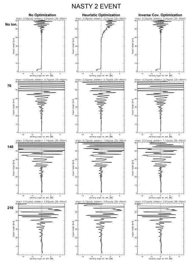
Figure B.1.3: Relative difference between retrieved and "true" bending angle. Event case: Nasty 2 event.
