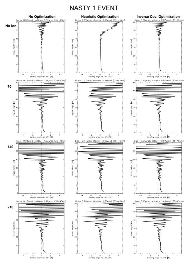
Figure B.1.2: Relative difference between retrieved and "true" bending angle. Event case: Nasty 1 event.
