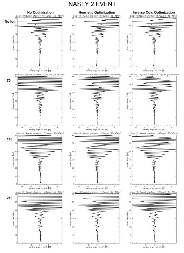
Figure A.1.3: Relative difference between retrieved and "true" bending angle. Event case: Nasty 2 event.
