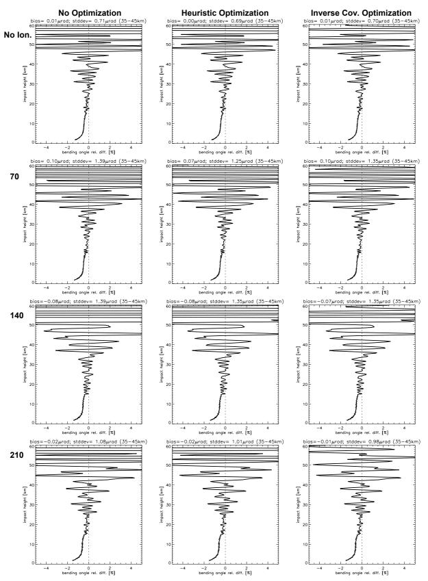
Figure A.1.1: Relative difference between retrieved and "true" bending angle. Event case: Nice event.
