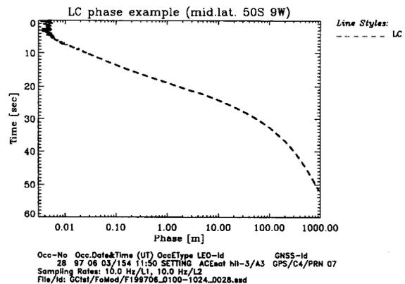
**Fig. 10.** Typical example for simulated ionosphere-corrected excess phase path profiles.
