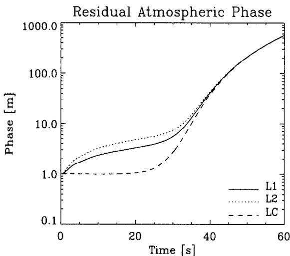
Fig. 3. Measurements of residual phase delay for the L1 and L2 GPS signals as well as the ionosphere corrected path delay LC are shown. The data are from occultation event no. 7 on October 21, 1995, 03:35 UT, located at 71°S and 151.6°W.
