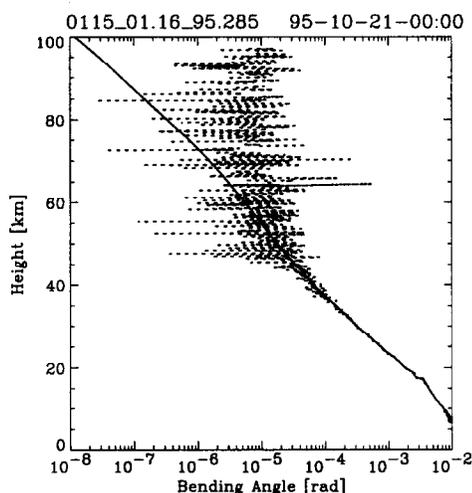
**Fig. 5.** Bending angle profile calculated from GPS/MET phase measurement data (dotted line) for occultation event no. 115 on October 12, 1995, located at 1.1°S and 51.9°W. The profile denoted by the solid line is obtained by combination with a co-located MSISE-90 model bending angle profile (from Steiner *et al.*, 1999).
