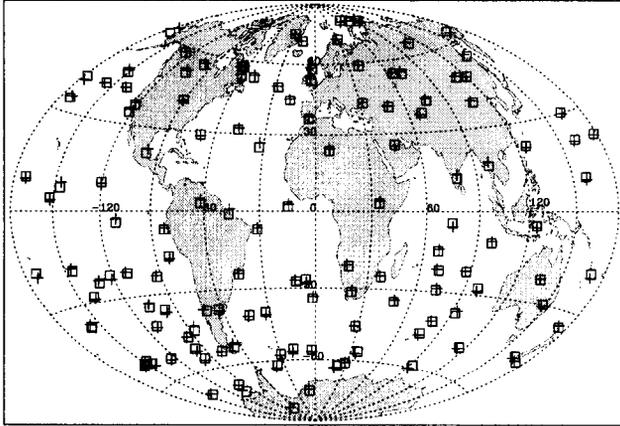
Fig. 2. One observational day (October 20, 1995) of the GPS/MET experiment showing 131 occultation events. Each individual event is visualized by the tangent point location of a high-altitude (mesospheric) occultation ray (center of square symbol) and of the bottom-most (tropospheric) ray (plus symbol).
