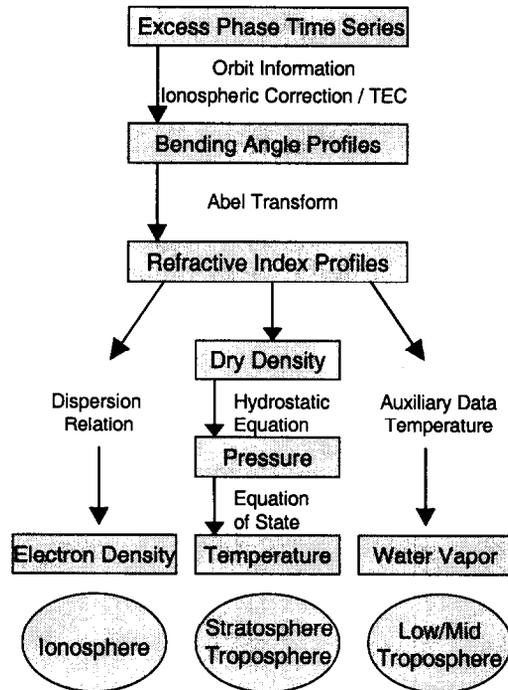
Fig. 4. Scheme summarizing the steps for the derivation of atmospheric and ionospheric parameters from radio occultation measurements (adapted from Høeg *et al.*, 1995).
